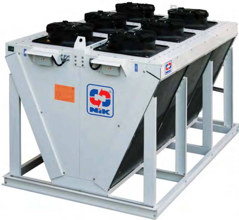
V-type dry coolers NDC-V Capacity range 15 up to 500 kw NO. of fans 2 ~10 fans Fan diam. 630, 710, or 800 mm
