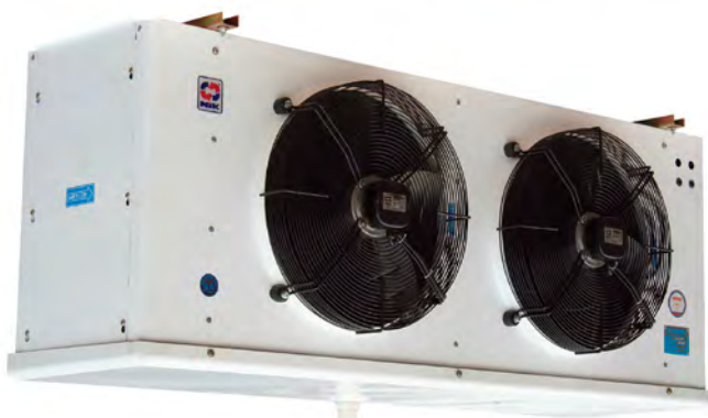
Horizontal unit cooler NBC-H Capacity range 1.7 to 76.7 kW Fan diameter 350, 400, 450 or 500 mm NO. of fans 1, 2, 3 or 4 fans Fin spacing 4, 6 or 8 mm
