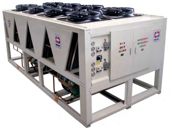
Air cooled liquid chiller(Reciprocating) NCA-R Cooling capacity range 20 to 120 ref. tons Power input range 18 to 108 kW
