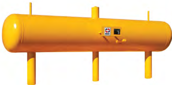
Ammonia surge drum NSD Diameter range up to 1 m Length range up to 3 m Working pressure range up to 20 bar
